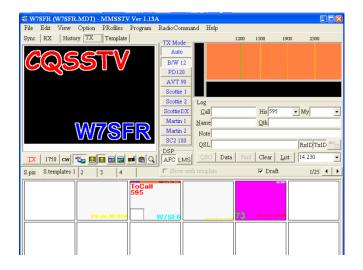
To change the tone frequency, right click on the tone frequency button, and enter the new tone, then hit OK to return to the main screen. You should see the new frequency posted in the button.
